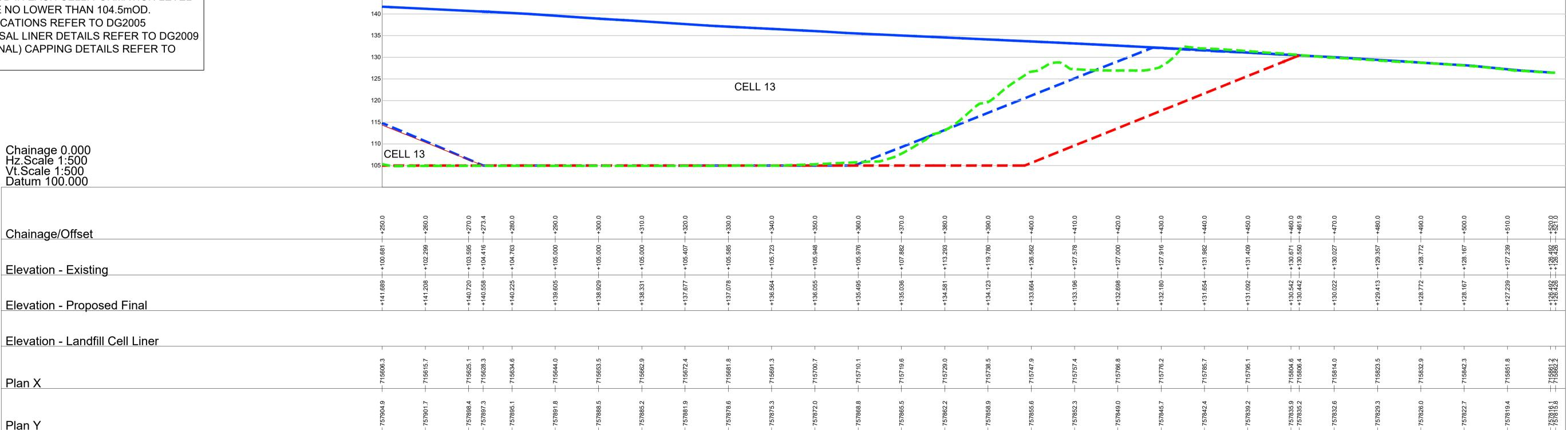
SECTION 4-4: LONG SECTION OF PROPOSED CELLS & EXISTING LEVELS
